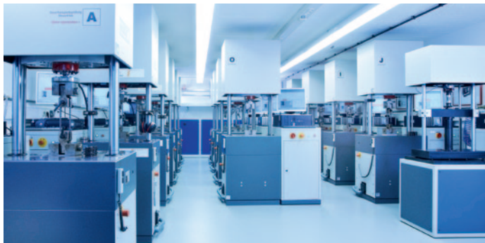
More than 15 pulsers are available for testing dynamic fatigue strength according to different testing methods
