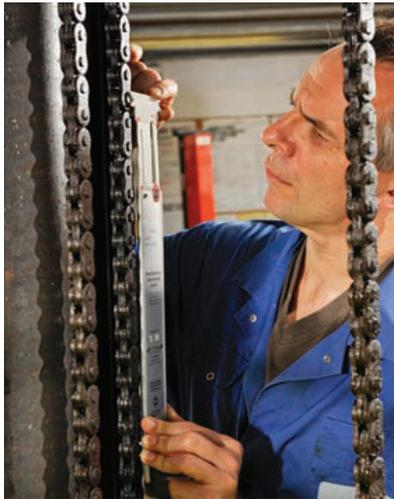
In the United States for example, Carolina Handling - part of the Raymond Truck Sales and Servicing Network - has recently equipped each of its 200 mobile forklift field service technicians with an FB chain wear gauge.
